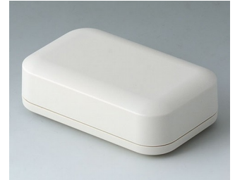
A9423107 EVOTEC 100, Vers. I ASA+PC (UL 94 V-0) gris blanc RAL 9002 100x62x31mm IP 65 opt., IP 40
