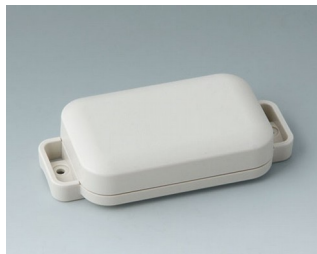
C3204107 EASYTEC 80 ASA+PC (UL 94 V-0) gris blanc RAL 9002 101x50x22mm IP 65 opt., IP 40
