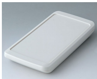
B5403307 SLIM-CASE M, Vers. III ASA+PC (UL 94 V-0) gris blanc RAL 9002 148x74x19mm IP 65 opt., IP 40
