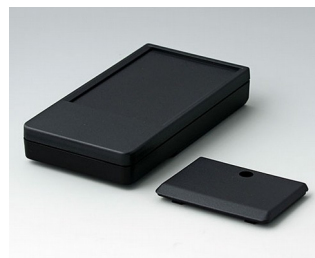
A9072119 DATEC-POCKET-BOX L ABS (UL 94 HB) noir RAL 9005 120x65x22mm IP 54
