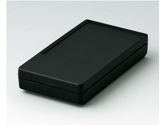
A9070119 DATEC-POCKET-BOX S ABS (UL 94 HB) noir RAL 9005 85x46x16mm IP 54
