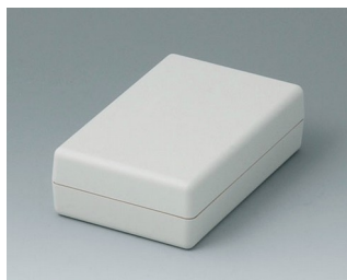
A9406331 BOITIER COQUILLES G 110, Vers. I ABS (UL 94 HB) gris blanc RAL 9002 72x114x33mm IP 65 opt.
