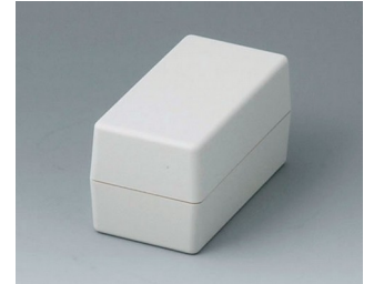
A9404441 BOITIER COQUILLES G 85, Vers. I ABS (UL 94 HB) gris blanc RAL 9002 45x85x45mm IP 65 opt.
