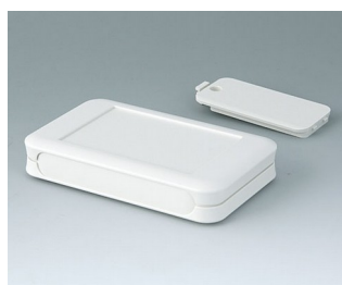
A9051117 SOFT-CASE M ABS (UL 94 HB) gris blanc RAL 9002 65x105x19mm IP 40
