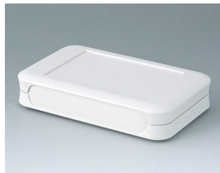
A9052107 SOFT-CASE L ABS (UL 94 HB) gris blanc RAL 9002 73x117x24mm IP 54 opt., IP 40
