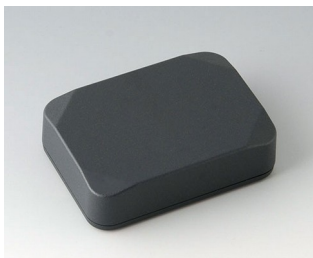
B1824218 MINI-DATA-BOX E50, haute ASA+PC (UL 94 V-0) gris anthracite RAL 7016 70x50x20mm IP 65 opt., IP 40
