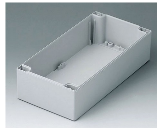
C2122402 Coquille 120, sans joint PC (UL 94 HB) gris clair RAL 7035 240x120x60mm
