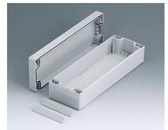
C2008242 ROBUST-BOX 80 LARGE, Vers. II PC (UL 94 HB) gris clair RAL 7035 240x80x60mm IP 66
