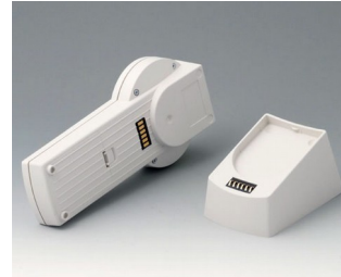
A9076157 JEU: DATEC-CONTROL XS, Vers. I, socle... ABS (UL 94 HB) gris blanc RAL 9002 200x94mm IP 65 opt.
