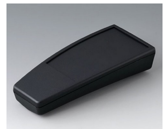
A9068219 SMART-CASE XL, Vers. II PMMA (IR) (UL 94 HB) noir RAL 9005 168x74,4x35,4mm IP 65 opt., IP 40
