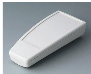
A9067117 SMART-CASE L, Vers. II ABS (UL 94 HB) gris blanc RAL 9002 140x62,7x30,5mm IP 65 opt., IP 40
