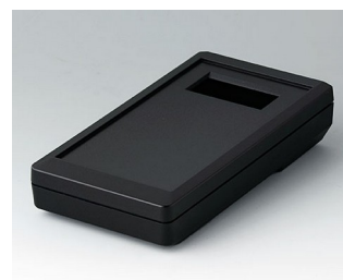
A9073419 DATEC-MOBIL-BOX S, Vers. IV ABS (UL 94 HB) noir RAL 9005 152x83x33,5mm IP 65 opt.
